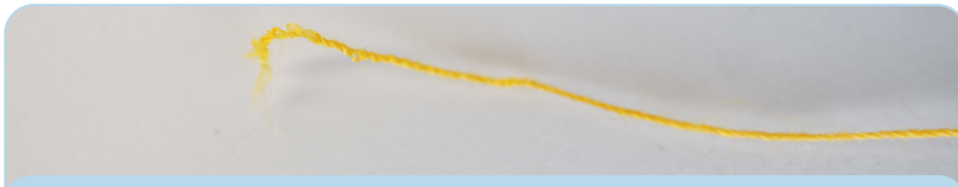
Tension Break: too much tension caused the thread to snap.
